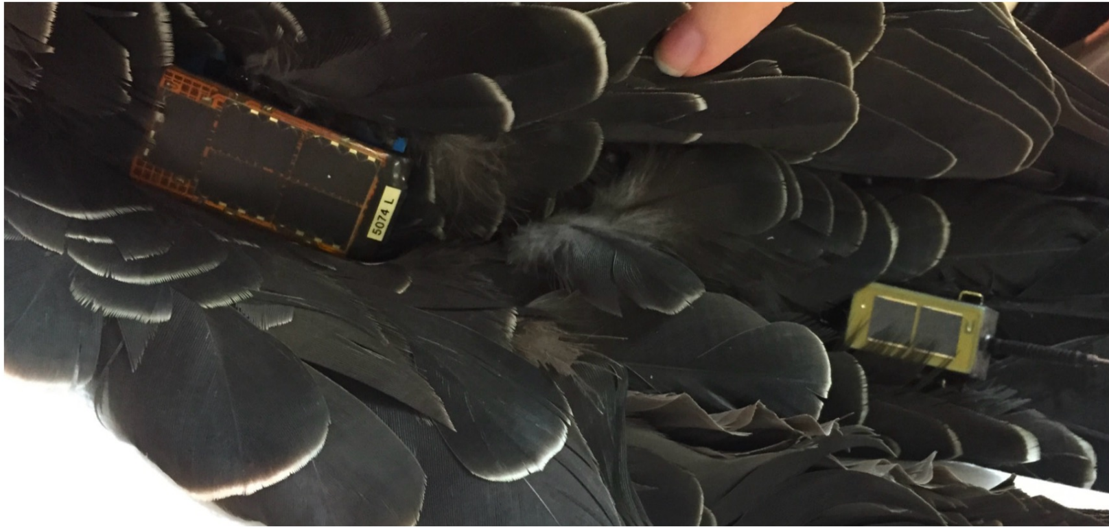
Figure 2. Double-mount of satellite and GPS tags dorsally on a black-cockatoo: Microwave Telemetry PTT-100 (at right) attached to dorsal aspect of central rectrices, and UvA-BiTS (5CDLe) (at left) attached to the feathers on the back of a Carnaby's Black-Cockatoo. Photo: Lian Yeap & Jill M. Shephard
